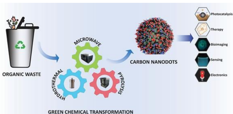
Scheme 1 Schematic summarizing the transformation of wastes to functional carbon nanodots.
