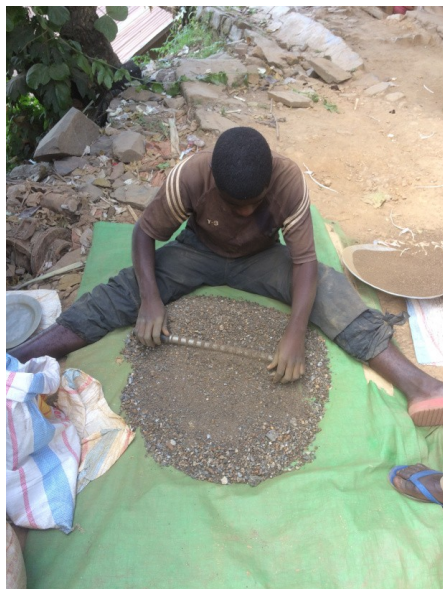
Magnetic pre-treatment of samples specifically used to eliminate iron oxide particles
